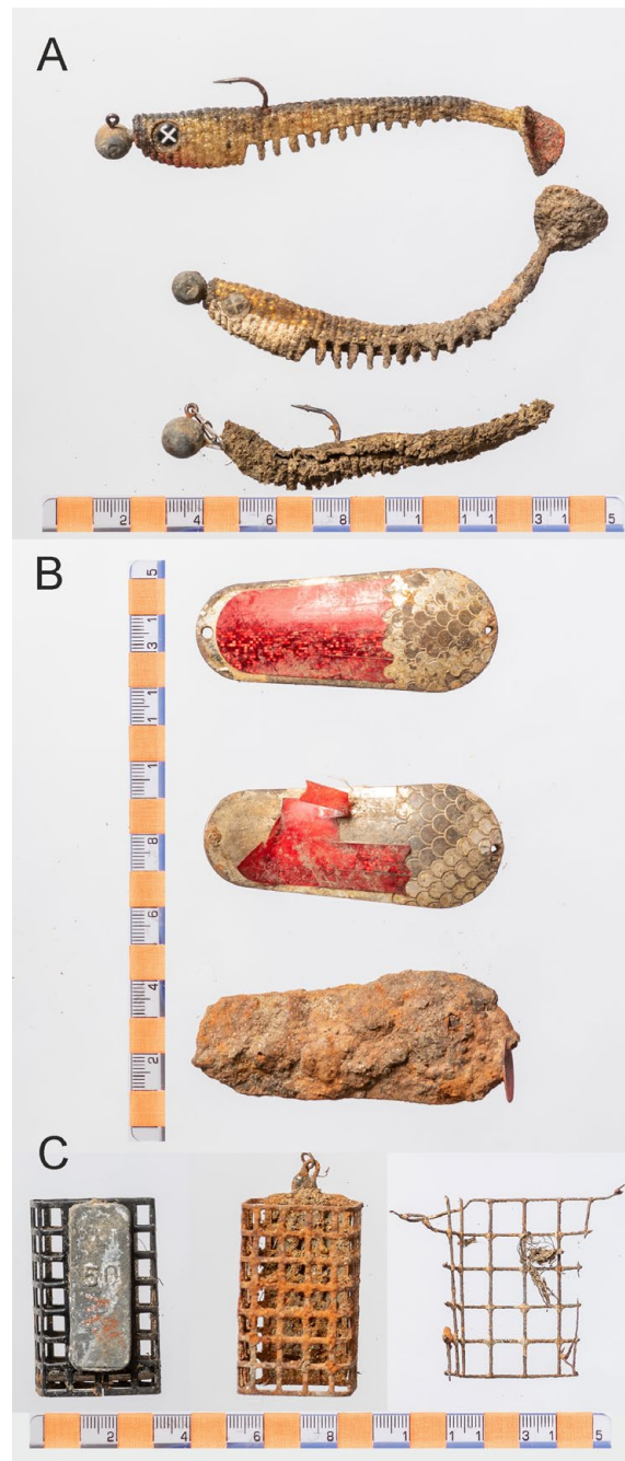
Figure 3. Different stages of degradation of (A) soft bait and (B) hard bait as well as (C) feeder baskets found in Lake Eixendorf.
